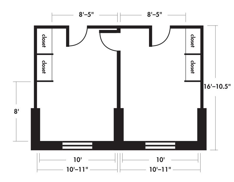
Corner room floor plan rooms 01 and 02 with 22 and 23 mirror images on each floor
